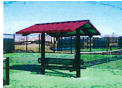
EXHIBIT 1: 8' X 8' GABLE END STEEL FRAMED MINI SHELTER
