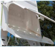
Global M4 includes a 5.6 cu/yd hopper capacity compared to 4.5 cu/yd for competitive machines resulting in more curb miles swept between dump cycles. With near Full Useable Capacity, 12,000 Lift Capacity, and the Optional Elevator and Hopper Wash Out System, Global M4 is Affordable, Reliable and Innovative.
