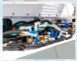
IT'S ALL IN THE OPEN Hydraulic Hoses are NOT hidden in the frame of the sweeper, while all Manifolds and Filters are located in a central location.
