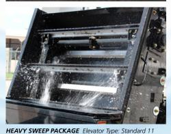
Flight squeegee with replaceable corded rubber tips; Continuous molded rubber belts combined with standard Heavy Sweep Package make **Global M4** the logical choice for sweeping heavy debris such as road millings, sand and gravel up to **3-Tons per-Minute**. That is one ton of sand every 20 seconds! Standard leaf gate system assists in picking up large debris, bottles, large branches and leaves.
