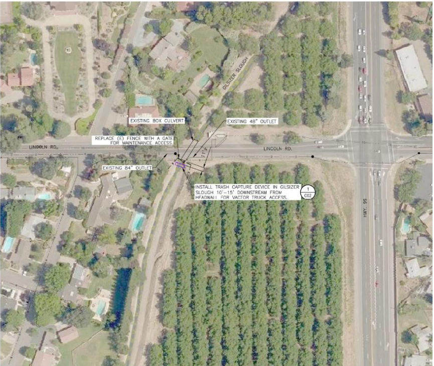
GILSIZER SLOUGH AT LINCOLN ROAD TRASH CAPTURE
